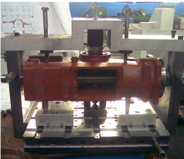
Figure 12 Photo image of the fixture used in the first machining process
