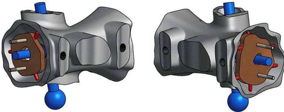
Figure 5 3-D model of workpiece with built-in mandrels on internal support elements
